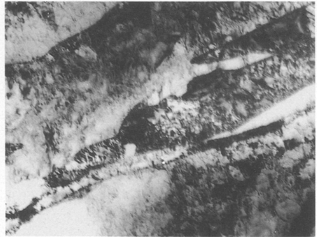
Figure 4 An electron micrograph of the as-quenched sample showing the lath martensitic structure prior to ageing.
