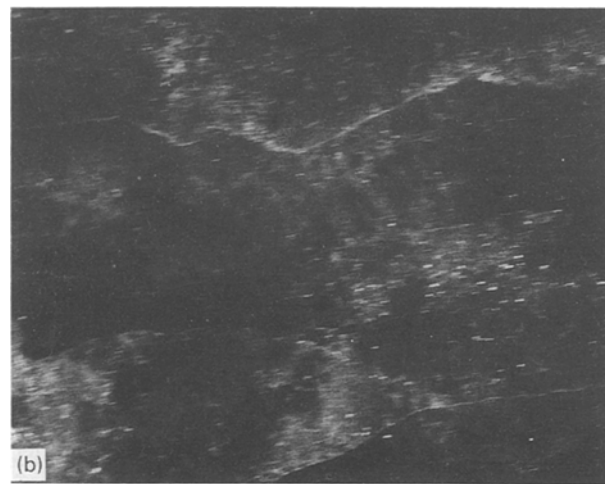
Figure 15 A transmission electron micrograph of base metal after ageing at 525°C for 3 min. (a) Bright-field image and (b) diffraction pattern. Precipitates are fcc copper and they are coherent with the bcc matrix. (●) [\bar{1}11]\ bcc , (■) [011]\ Cu .
